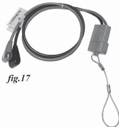
1. Connect the winch leads, tagged "To Motor", to the contacts on the winch motor as shown. [winch leads photo] Be sure the rubber caps cover the connections well to prevent water entry. The red lead should be connected to the positive (+ upper) terminal on the winch, and the black lead connected to the negative (- lower) winch terminal.
