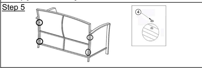
Fully tighten all bolts at all joints, then cover the four Backrest Bolts with Nut Cap ( 1 ).
