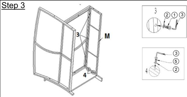
Place the Front Panel(M) as pictured above and affix to Seat (L) and Right Armrest(C). Attach Front Panel(M) to Seat(L) using Hardware(125) with Allen Key(3) as shown in Picture 3 and Picture 4. **Do not fully tighten the bolts at this stage.**
