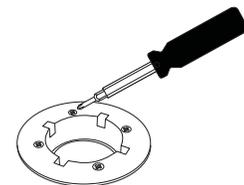
**14** Tighten all four Phillips head wing screws evenly until drain is secure in pan. 20 Inch pounds maximum!
