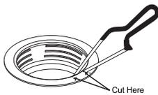
**8** Remove shower drain from pan. Clean shower surface around drain hole, above and below the pan to insure proper seal and unrestricted wing movement.
