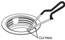
**5** Once horizontal flange is cut, use flat blade screwdriver to pry on 1" flange to break free from shower pan.
