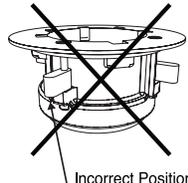
**13** Insert drain into shower pan and press evenly over 2" drain pipe. Once drain has made contact with shower pan, hold firmly in place. Inspect pipe riser to ensure full contact with O-ring seal.
