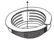
**4** Continue cutting horizontally through drain flange to weaken it, but not deep enough to damage pan.
