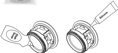
**10** Apply liquid dish soap to drain O-ring as lubricant.
