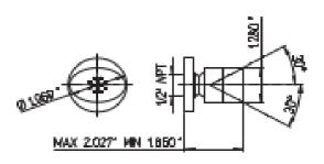
Novello 3-body jets 30 degree rotation 2.0 maximum flow rate each
