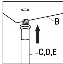
**NOTE:** Start with the side of the light fixture (A) that has power cables and feed the power cables through the downtube assembly (C,D,E). Repeat with the other downtube assembly (C,D,E) (minus the power cables).
