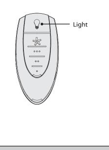
Quickly press the Light button to turn the lights off and on. Hold the Light button to raise and dim the light level.
