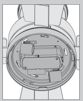
Align the keyhole slots in the light kit housing with the two screws. Make sure all the wires from the fan and the light kit are snug inside the center of the light kit, not pinched in between the upper switch housing and the light kit or hanging out of the sides.
