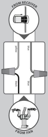
Using the orange wire connectors from the  $\bigstar$  hardware bag:
