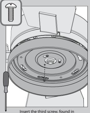
Insert the third screw, found in the  $\equiv$  hardware bag, into place and then tighten all three screws.
