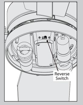
To switch the direction of air flow, remove the globe assembly and move the reverse switch to the opposite position. Reinstall the globe assembly.
