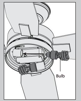
Install a light bulb in each socket. When necessary, replace with bulbs of the same wattage.
