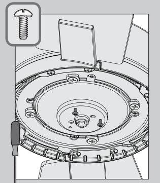
Screw two housing assembly screws
