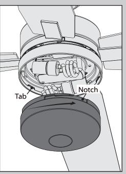
Position the notches in the outer rim of the globe so they line up with the tabs on the inside surface of the light fixture rim. Carefully lift the globe up inside the light fixture as far as it will go. Rotate the globe in a clockwise direction until it is held tightly in place by the three tabs.
