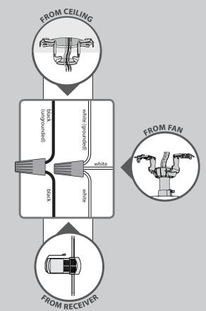
Turn the splices upward and push them carefully back through the hanger bracket into the outlet box. Spread the wires apart, with the grounded wires on one side of the outlet box and the ungrounded wires on the other side of the outlet box.
