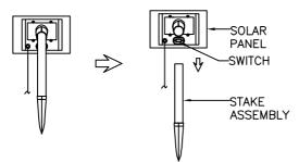
2.) Remove (4) screws from back of solar panel with screwdriver (not included).
