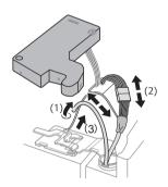
4 Rotate the hinge lever counterclockwise (1). Lift the top hinge (2) free of the hinge lever latch.
