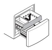
Remove the Durabase basket from the rails. Remove the screws from the rails at both ends.
