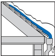
Water from melting snow over the heated portion of the house runs down the roof. It freezes at the cold eave and an ice dam begins to form preventing drainage.
