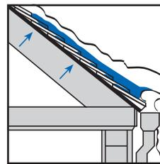
Grace Ice & Water Shield HT resists this leakage because of the seal around the fasteners, ability to make watertight laps, and the membrane's bond to the deck.
