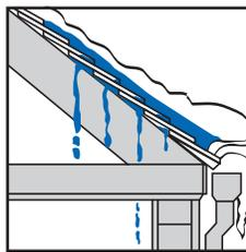
As the ice dam grows, water is trapped behind it and backs up under the shingles. Eventually it reaches the roof deck and leaks through, damaging the interior of the structure.
