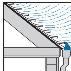
Grace Ice & Water Shield HT applied beneath the sloped roof covering helps prevent wind-driven rain from entering the structure.
