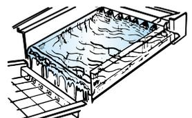
2. When the desired thickness is reached, the ice sheet is released and slides onto a cutter grid. The grid divides the sheet into individual cubes.
