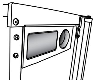
4. Using the arrow pointing to the alignment pin on the side of the filter and the arrow inside the control housing, align the alignment pin with the cutout notch and insert the filter into the housing.
