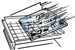
3. The water containing the rejected minerals is drained after each freezing cycle.
