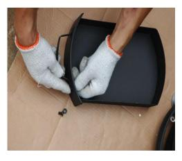
Assemble the ash drawer handle by installing 2 screws and nuts to the tray. Then slide it into place.
