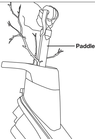
**⚠️WARNING!** Never put your hands into the hopper while the wood chipper + shredder is running. Always use the paddle supplied with your shredder to push items into the hopper.
