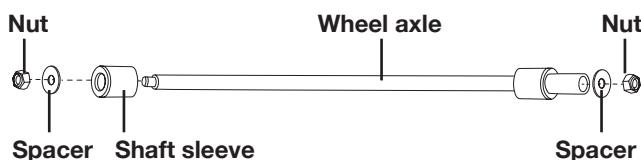
2. Insert the wheel axle into the shredder stand assembly, and re-assemble the shaft sleeve and the support cover (Fig. 2).
