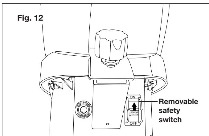
3. To power the wood chipper + shredder off, push the removable safety switch to the OFF position. To disable the machine, remove the safety switch completely (Fig. 13).
