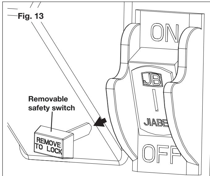
**NOTE:** As a safety precaution, the removable safety switch can be removed when you are not using the wood chipper + shredder to prevent children from starting it accidentally. The unit cannot be started when the safety switch is removed. Make sure to replace the removable safety switch before operation.
