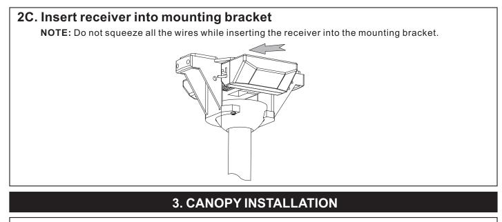
Note: Two screws are pre-installed on mounting bracket for canopy installation.
