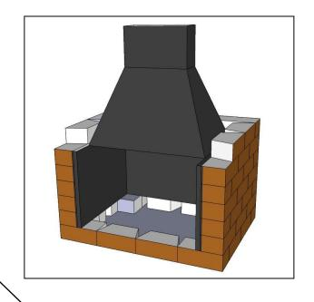
**Step 9**: Install row 7 of blocks (2 corners, 6 garden blocks). Start with a corner block as shown and continue around the rectangle making slight adjustments as needed. Using a tape measure or level, ensure the blocks are stacked vertically. Once the blocks are level and in place, proceed to step 10. The figure on the left is illustration of block placement. The figure on the right shows installation through step 9.
