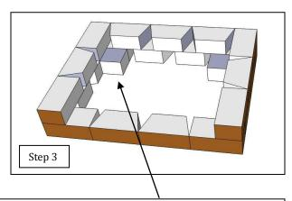
**Step 3**: Install row 2 of blocks (4 corners and 5 garden blocks). Place the 2 blocks with an "X" into the back corners. Next, place the first corner block on top of the bottom row staggering the intersection of two blocks on the row below. Continue around the rectangle making slight adjustments as needed so that the edge of the blocks fit tightly together. Once the blocks are level and in place vertically, proceed to step 4.
