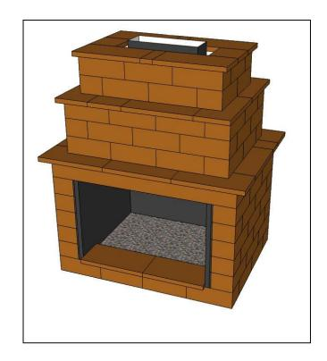
**Step 19**: Install hearth  $(1 - 11.5" \times 23.5" \text{ and } 1 - 11.5" \times 21.5" \text{ tile})$ . Place the 2 pieces of tile in between the sides of the steel insert on the bottom row of blocks. The amount of overhang to the front can be as desired. Once the tiles are in place, remove one by one and glue to the blocks below. Place approximately 6" of gravel in the bottom of the fire place. Installation is complete.
