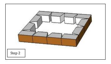
**Step 2**: Install row 1 of blocks (4 corner and 8 garden blocks). Lay out the blocks as shown measuring diagonally corner to corner to ensure a square base. Level the blocks from front to back and side to side (this applies to all steps). Blocks may need to be shifted slightly in order to get a tight fit between all the blocks on the first course.
