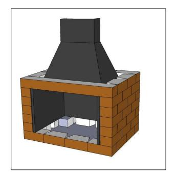
**Step 10**: Install the lentil. Set the lentil in place as shown above. Once it is level and in place, remove it and glue to the blocks below. Remove the blocks placed in step 9 (row 7) one by one and glue to the blocks below. The figure on the left is illustration of block placement. The figure on the right shows installation through step 10.
