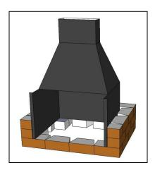
**Step 4**: Install the steel insert. Place the steel insert into the fireplace base with the back of the insert resting on the 2 (X) blocks in the back corners. There will be a gap between the blocks and the insert of approximately 1.5" to 2". Now ensure the blocks in row 2 are level, remove them one by one and glue to the blocks below.
