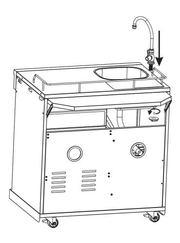
6. Remove the sink (Part No. 5) and then attach the detergent bottle (Part No. 4) on the top panel as shown, replace sink after detergent bottle assembly.
