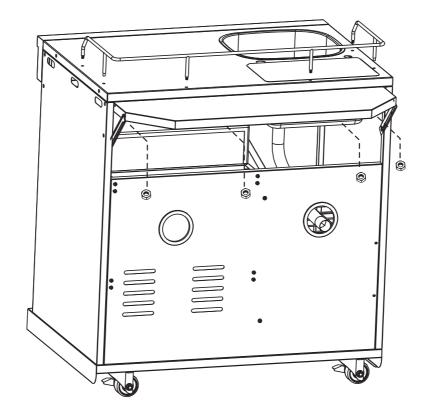
5. Assemble the tap (Part No. 2), and then screw into the quick water connector (Part No. 3).
