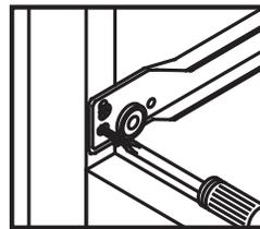
3. Tighten a #8 x 5/8" screw in the hole to fix the drawer glide in place.
