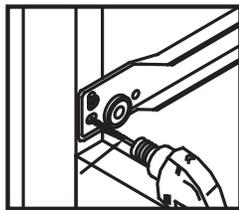
2. Drill 1/8" DIA. pilot hole in the second screw hole.
