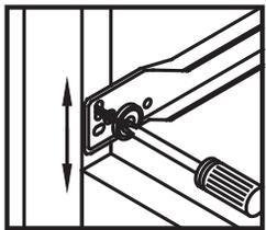
1. Loosen screw and make vertical adjustments.
