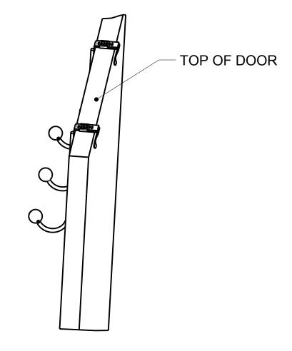
Slide open the adjustable brackets to fit over door.
