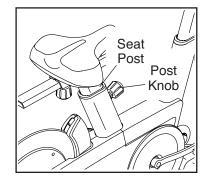
post knob. Make sure that the post knob is engaged in an adjustment hole.
