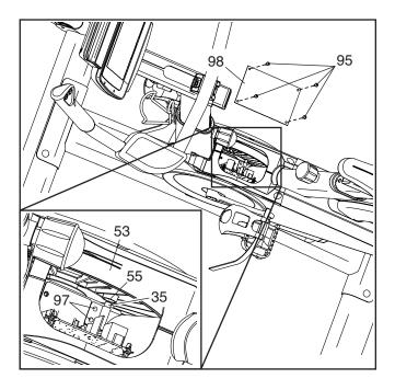
Next, rotate the Crank Pulley (53) until a Pulley Magnet (55) is aligned with the Reed Switch (35). Slide the Reed Switch slightly toward or away from the Pulley Magnet. Then, retighten the #8 x 19mm Tek Screws (97).
