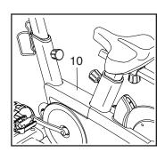
Next, remove the four #8 x 1/2" Screws (95) and the Electronics Shield (98). Then, locate the Reed Switch (35), and **loosen** the two #8 x 19mm Tek Screws (97).
