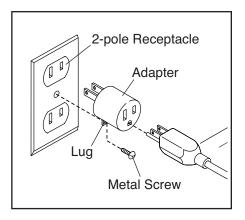
The lug or wire extending from the adapter must be connected with a metal screw to a permanent ground such as a properly grounded outlet box cover. Some 2-pole receptacle outlet box covers are not grounded. Before using an adapter, contact a qualified electrician to determine whether the outlet box cover is grounded before using an adapter. The temporary adapter should be used only until a properly grounded outlet can be installed by a qualified electrician.
