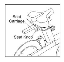
seat knob. Make sure that the seat knob is engaged in an adjustment hole.
