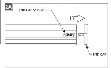
Loosen the two end cap screws on each end of the fixture and remove the standard end caps.
