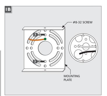
Attach the mounting plate to the electrical box using the two #8-32 screws provided.
