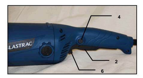
This tool is started by depressing the safety (6) and engaging the switch (2). The tool is stopped by releasing the switch (2).
