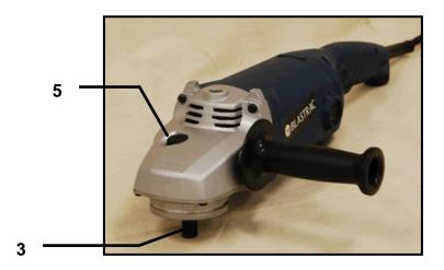
To lock the spindle from rotation, press and hold the spindle locking button (5). Turn the spindle shaft (3) until the shaft locks in position. To release, simply let off the locking button (5). The shaft should turn freely.
