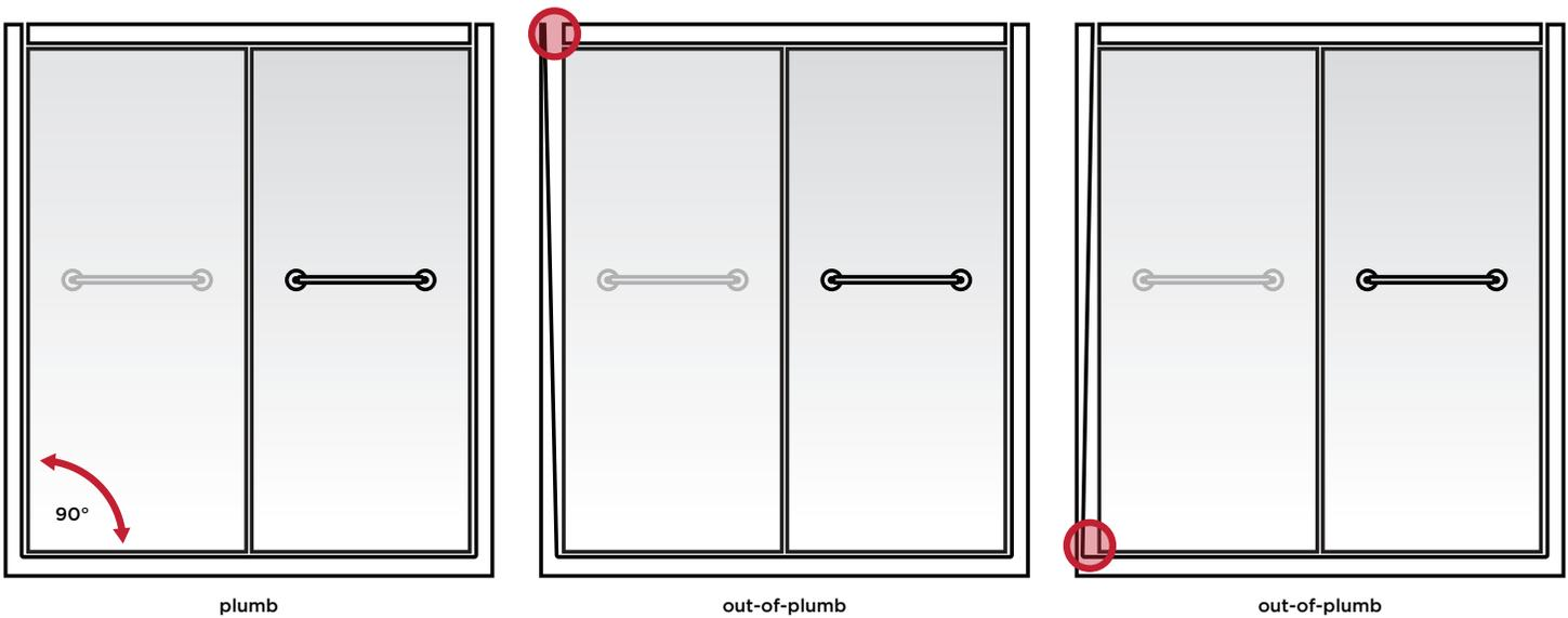
Most **Delta Shower Doors** are designed to accommodate out-of-plumb conditions up to 3/8". If your shower environment is out-of-plumb, simply adjust the placement of the roller to lower or raise the glass.
