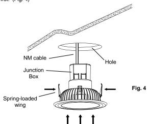
Continue inserting the EasyUp™ trim into the hole, while continuing to squeeze the spring-loaded wings. When the wings reach the hole edge, release them and push up the EasyUp™ trim until both wings flip down onto the ceiling surface. (Fig. 5) The decorative ring of the EasyUp™ trim should be flush against the ceiling surface.
