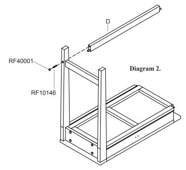
Step 2 : Attach Back Support Bar (D) to the leg frame using Long Bolt (RF10146) secure screws tightly by using Allen Key (RF40103).
