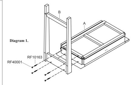
Step 1: Turn Table Top (A) upside down on soft surface to protect from scratching, attach Right Leg Frame (B) using Short Bolt (RF10163) secure all screws tightly by using Allen Key (RF40103).
