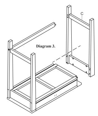
Step 3 : Assemble Left Leg Frame (C) by repeating step 1&2 as shown Diag.3.
