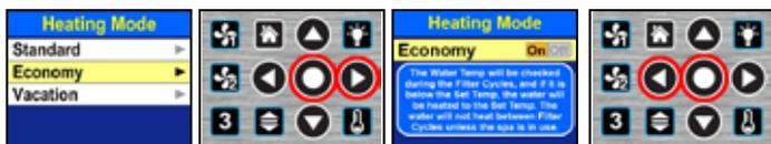
The Default Heating Mode is Standard Mode. Move Down and Touch Right or Select to Open the Heating Mode Set Menu. To change to this Heating Mode, Touch Select, or to Exit back, Touch Left.
