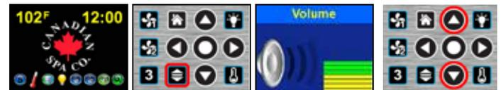
From the Home Screen, Touch the Audio Volume Button to open the Volume Control Menu. The Audio Volume Level Menu is Open, indicating the Volume Level.
