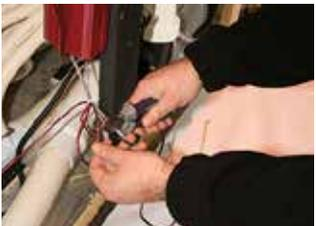
**STEP 5** - Cut Black/Red and Red wires on amplifier wires.
