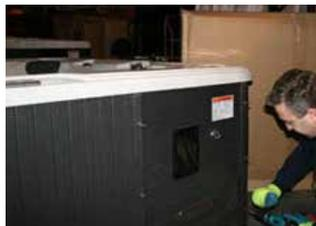
**STEP 1** - Unscrew side panels to access pump on the side with air vent and the MP3 Player housing
