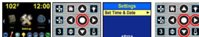
To Set Time & Date, in Navigation Mode, with Settings Highlighted, Touch Select to Open the Settings Menu. Scroll Down , and with Set Time & Date Highlighted, Touch Select or Right to Open the Set Time & Date Menu.
