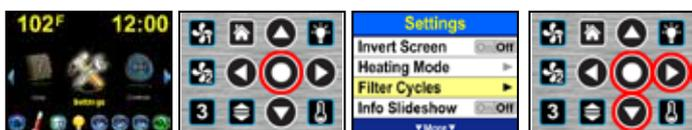
To Set the Filter Cycles, in Navigation Mode, with Settings Highlighted, Touch Select to Open the Settings Menu. Scroll Down, and with Filter Cycles Highlighted, Touch Select or Right to Open the Set Filter Cycles Menu.
