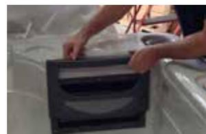
**Step 1.** Remove the filter cover by sliding up the front plate
