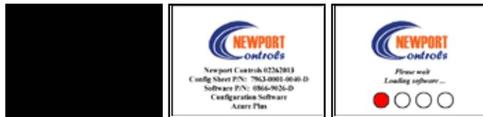
It will take 3 to 4 minutes for the Software to Load and Control System to Initialize. After the Power is ON, the Control Panel Button Backlighting will turn ON, but the Display Screen will remain Black for about 20 seconds. Then, for the next 20 seconds, there will be a Screen that shows the Serial and Part Numbers. At about 40 seconds after the Power is ON, there will be a Screen indicating that the Software is Loading.
