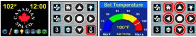
To Adjust the Set Temperature, at the Home Screen, Touch Temp to Open the Set Temperature Menu. On the Set Temperature Menu, Touch the Up and Down Buttons to Raise or Lower the Water Set Temperature in 1°F or 0.5°C increments. Touch Left to go to the lowest Set Temp of 70°F (21.0°C), or Touch Right to go to the Highest Set Temp of 104°F (40.0°C). Then Touch Back Home to Exit. To Set a Temperature higher than 104°F (40.0°C), see "Set Over Temperature".
