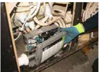
**STEP 5** - Unscrew Control pack cover using a Phillips screwdriver
