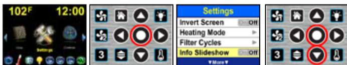
To turn On the Info Slideshow, in Navigation Mode; with Settings Highlighted, Touch Select to Open the Settings Menu. Scroll Down, and with the Info Slideshow Menu Bar Highlighted, Touch Select to Start the Info Slideshow.
