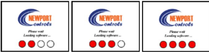
The four White Progress Dots at the Bottom of the Screen will advance about every minute until all four Dots are Red.
