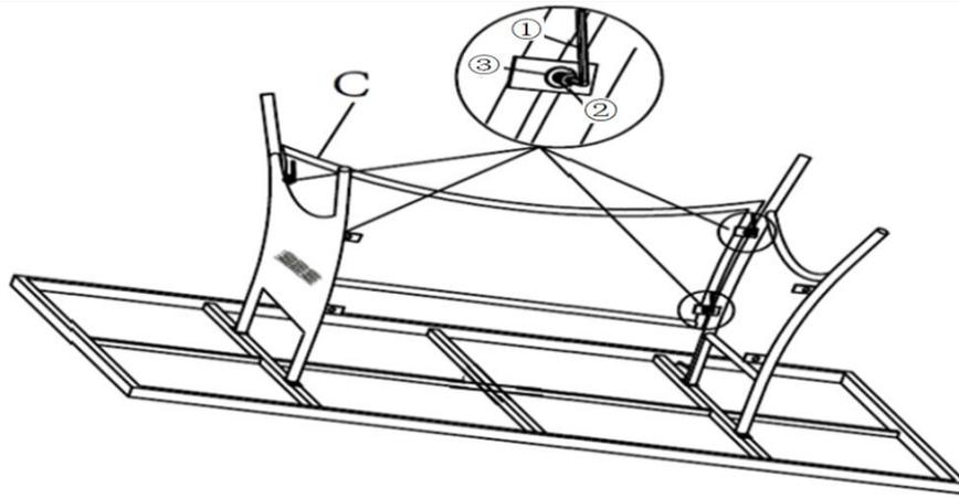
Attach Leg Support Panel(C) between Leg Panels(B) using Bolt(2) and Washer(3) with Allen Key(1) as shown in the picture above.
