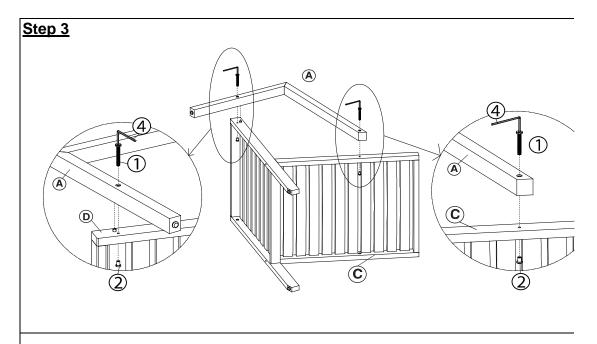
Attach Right Armrest (B) with the assembled frame in step 2 as shown in picture. Then secure the Right Armrest (B) with the assembled frame by using Bolts (1), Slevee nut (Allen Key (4)).
