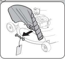
Check the mower deck for a shipping brace that may be holding the chute deflector upward for shipment. If the brace is present, it must be removed before operating the tractor. Holding the chute deflector fully upward, remove the shipping brace. Lower the chute deflector and discard the shipping brace.
