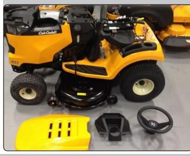
Un-crate the rider and lay out the hood topper, dash cover and steering wheel for easy access. Watch for staples when rolling the tractor off the pallet.
