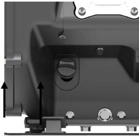
Figure 1 – Unscrew the Dipstick Cap
