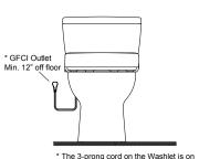
1 he 3-prong cord on the Washiet is on the left side and is 3' long. The GFCI outlet needs to have 120V, 10amps.
