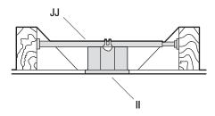
To hang your fan where there is an existing fixture but no ceiling joist, you may need an installation hanger bar (JJ) (not included) as shown above.
