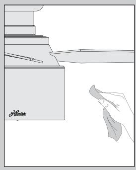
For cleaning the fan, use soft brushes or cloths to prevent scratching. Cleaning products may damage the finishes.
