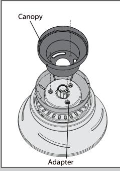
Place the canopy on the top housing. Ensure all four screw holes line up with the screw holes in both the top housing and the adapter.
