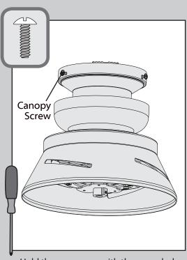
Hold the canopy up with the screw holes aligned. Partially install two canopy screws, found in the hardware bag, into the holes opposite the ceiling plate hooks.
