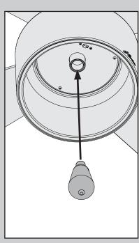
Install the bulb into the socket. When necessary, replace with bulb of the same type and wattage.
