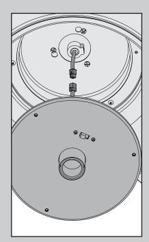
Connect the plugs from the fan and lower switch housing. Make sure to line up the colored markings on the connectors.
