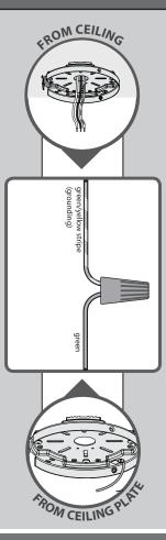
Turn the splices upward and push them carefully back through the hanger bracket into the outlet box. Spread the wires apart, with the grounded wires on one side of the outlet box and the ungrounded wires on the other side of the outlet box.
