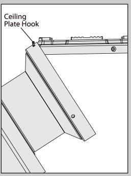
Place the slots over the ceiling plate hooks to hang the fan.
