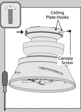
Partially install a canopy screw, found in the hardware bag, between the ceiling plate hooks. When all the holes are properly aligned, securely tighten all three canopy screws.
