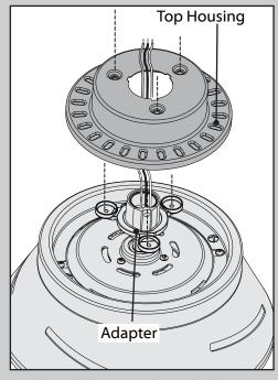
Thread the wires through the top housing. Place the top housing onto the motor housing so that the holes in the top housing lineup with the holes in the motor housing and the adapter.
