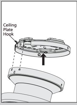
Raise the fan and align the slots in the canopy with the hooks on the ceiling plate.
