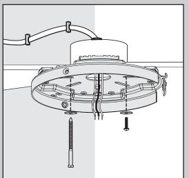
Use wood screws (included) when securing to support structure with approved electrical outlet box. Drill 9/64" pilot holes in support structure to aid in securing ceiling plate with hardware found in the  $\bigstar$  hardware bag.
