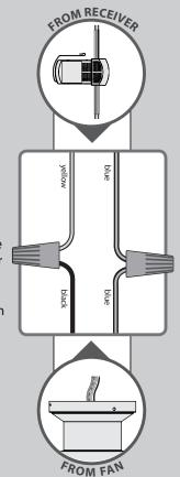
Using the orange wire connectors from the hardware bag, connect the black wire (ungrounded) from the ceiling to the black wire from the receiver.
