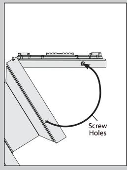
Swing the fan up to align the canopy screw holes with the mounting holes on the ceiling plate.
