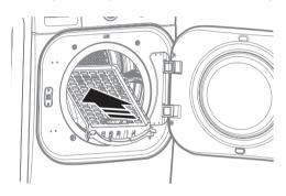
2. Make sure it is seated evenly on the edge of the inner door rim and resting flat on the inside of the dryer.
