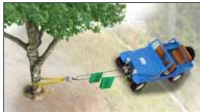
A typical double-line winch and pulley arrangement doubles winch capacity.
