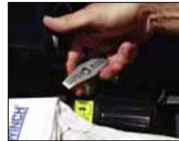
The Superwinch Thimble Protects wire rope from wear and tear, extends wire rope life.
