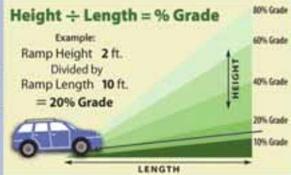
It's a common mistake to confuse the degree of the angle of a slope with the grade percent. Angle (degree) is a geometric measure. You must know the grade % to find the Rated Line Pull you need.
