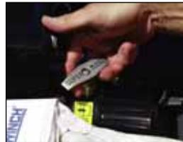
Solenoid housing on the EP12.5 and 16.5 is removable to allow custom remote mounting. Requires wiring kit, FN 2302283
