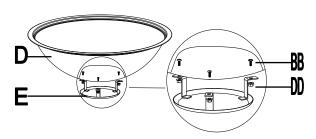
**Step 5:** Turn over the whole assembled piece. Place Fire bowl (D), Grate (C), Cooking grate (B) and Fire screen (A) in order. Use Poker (J) and PVC cover (K) as necessary.
