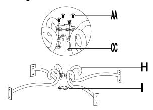
**Step 3:** Connect assembled Leg connector (H) and Leg (G) with bolt (AA) and washer (EE). **Tighen all bols here.**
