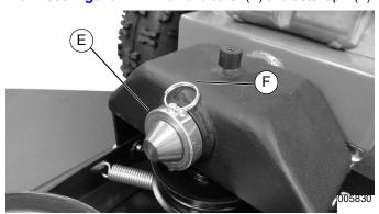
Figure 2-12. Detent Pin and Collar
