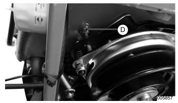
Figure 4-12. Anti-Rotation Bolt Location
