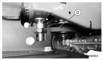
Figure 2-11. Belt Installed
