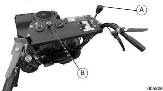
Figure 3-3. Wheel Speed Lever
