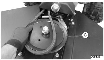
Figure 2-10. Removing Belt from Blade
