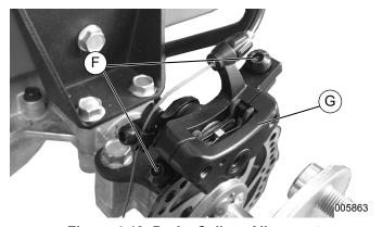
Figure 4-18. Brake Caliper Alignment
