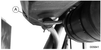
Figure 3-2. Fuel Shut-Off Valve
