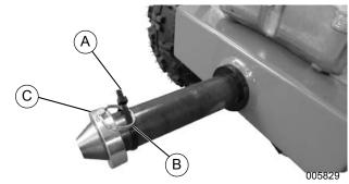
Figure 2-3. Detent Pin and Collar
