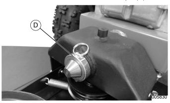
Figure 2-4. Detent Pin and Collar Installed
