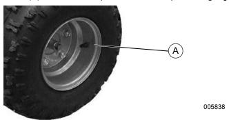
Figure 2-18. Valve Stem Location
