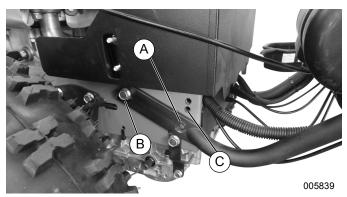
Figure 2-20. Handlebar Height Adjustment
