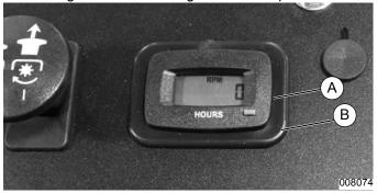
Figure 2-13. Maintenance Meter Installation
