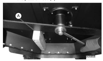
Figure 4-13. Mower Blade Removal
