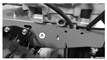
Figure 4-3. 18.67 HP Oil Drain
