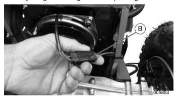
Figure 4-9. Clutch Connector
