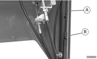
Figure 4-6. Traction Drive Cable
