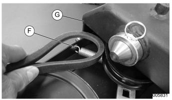
Figure 2-5. Belt Insertion Point
