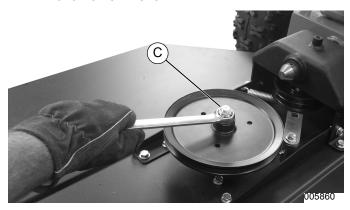
Figure 4-15. Blade Pulley Locknut
