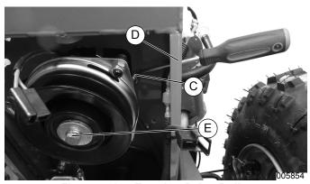
Figure 4-10. Traction Drive Pulley
