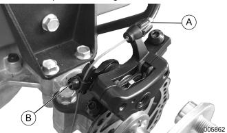
Figure 4-16. Brake Cable Adjustment
