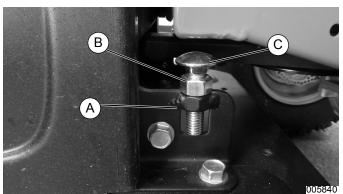
Figure 2-21. Carriage Bolt and Locknut
