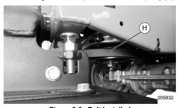
Figure 2-6. Belt Installed
