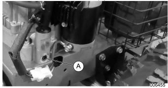
Figure 4-2. 16 HP Oil Drain
