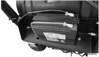
Figure 2-19. Connecting Battery Cable
