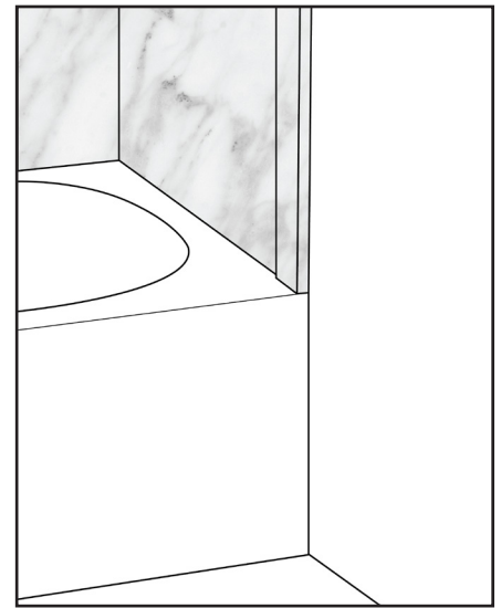
Vertical trims installed to top of tub
