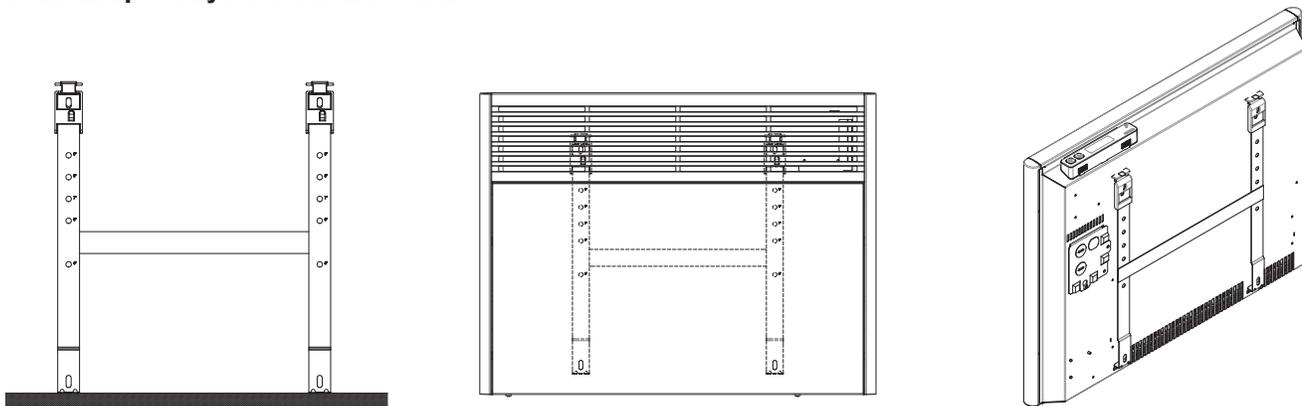
THE BOTTOM OF THIS UNIT MUST BE INSTALLED AT LEAST **4 INCHES (10.2 CM)** FROM THE FLOOR.
