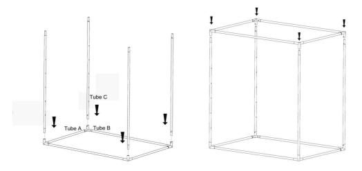
2. Insert four hooks in to the bottom holes of Tube C.
