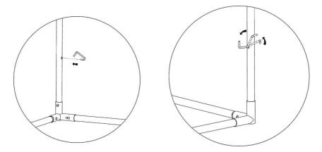
3. Hang the first support rack by using four hooks. Install the second support rack in the same manner. You may adjust the height according to your needs.
