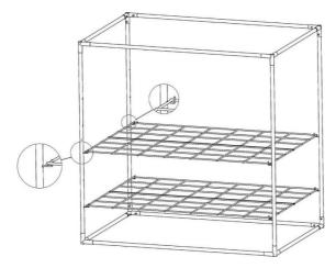
4. Open the Bedbug Toaster<sup>™</sup> and assemble it carefully over the outer structure. Put the items intended for heat treatment on the support racks.
