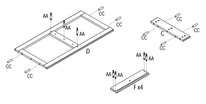
3 Locked cam bolt(AA) and attached wooden dowel(CC) to side panel(B)
