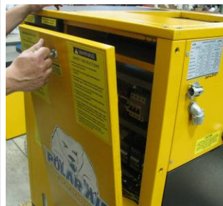
A. Using lock key, remove electrical panel from unit
