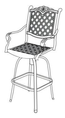
Make sure that the Chair Seat and the Chair Leg Base is fully and firmly attached together as one complete piece.
