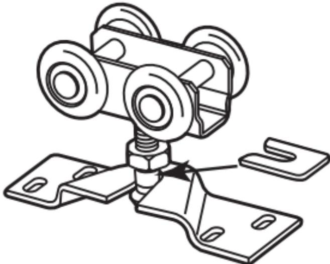
After door is hung, insert between bracket and nut; press in firmly to lock into place.
