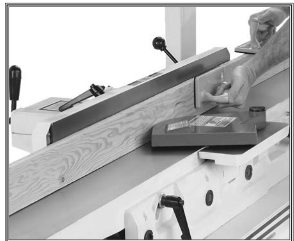
Figure 33. Typical edge jointing operation.
