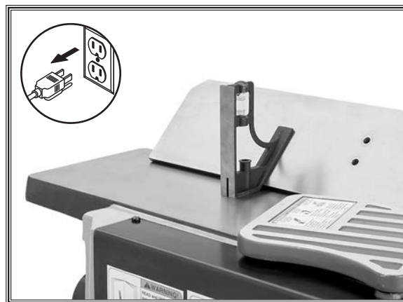
Figure 47. Checking the outward 45° stop.
