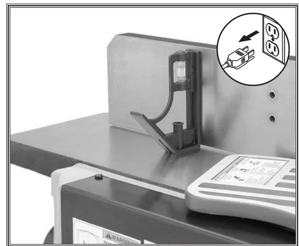
Figure 44. Checking the 90° stop.
