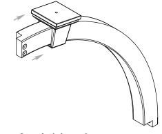
Note: There are Left and Right Arches. Make sure the pre-drilled holes are in line between the two arches.
