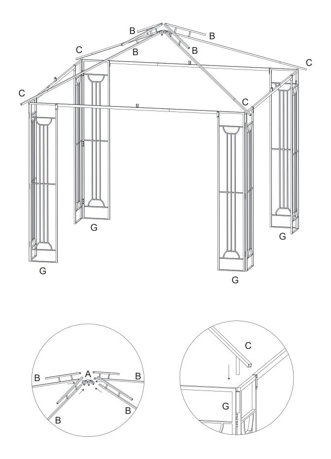
5. Insert Long Support Connecting Tube (B) into Center Connector (A) then insert them into the round tube of Door Screen (G) ;
