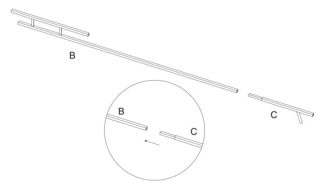
4. Insert Long Support Connecting Tube (C) into Long Top Bar Tube (B);
