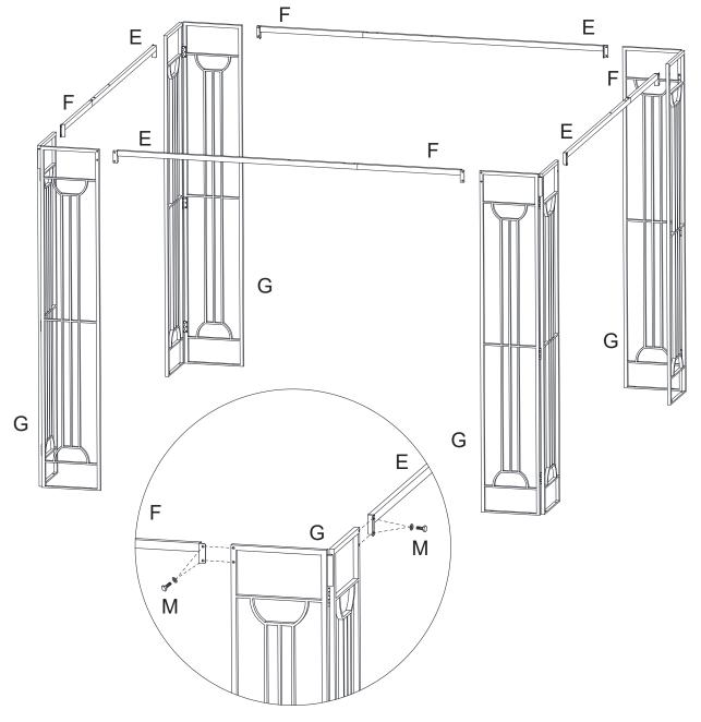
2. Fix the Well connected Short Cross Beam (F) and Long Cross Beam (E) with Screw (M) and Door Screen (G);
