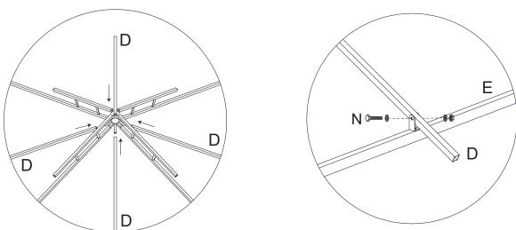
6. Insert Short Top Bar Tube (D) into Center Connector (A), then fix Short Top Bar Tube (D) with U-Shaped Connector (I) with Screw (N) ;
