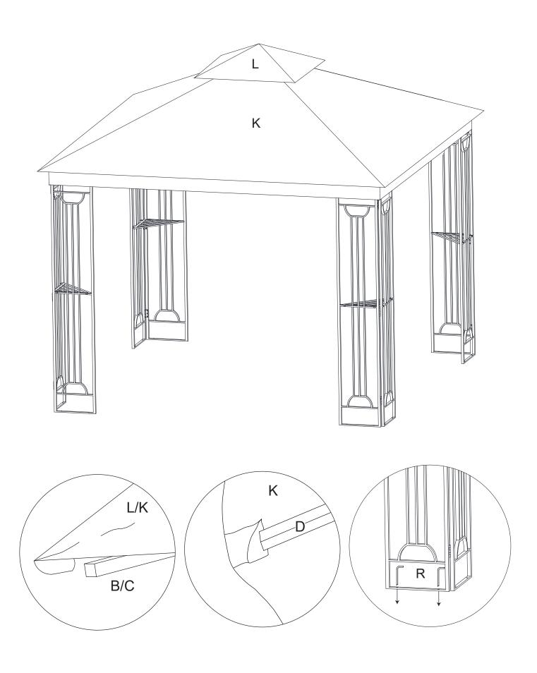
8. Put Big Canopy (K) and Small Canopy (L) on tope of Long Top Tubes (B/C) and Short Top Bar Tube (D), fix Door Screen (G) by Stake (R) firmly .
