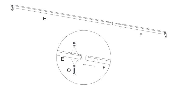
1. Insert Short Cross Beam (F) into Long Cross Beam (E) fasten tightly with Screw (O);
