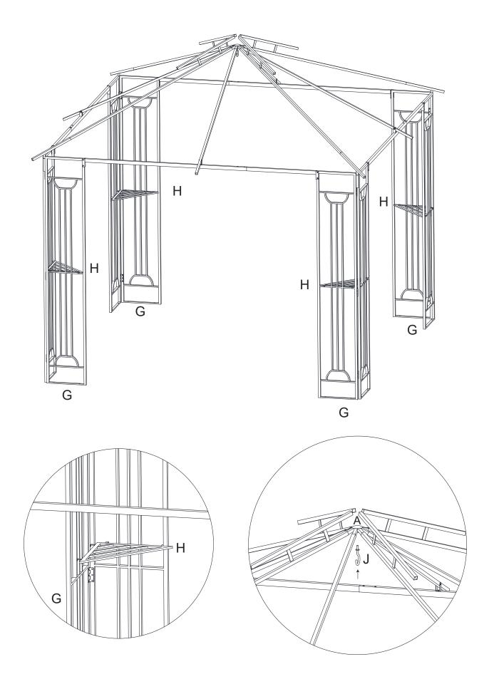
7. Put Triangle panel insert into Door Screen (G), fasten Hook (J) tightly into Center Connector (A) ;
