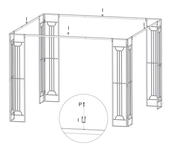
3. Fix U Shaped Connector (I) with Cross Beam (F)with Screw (P);
