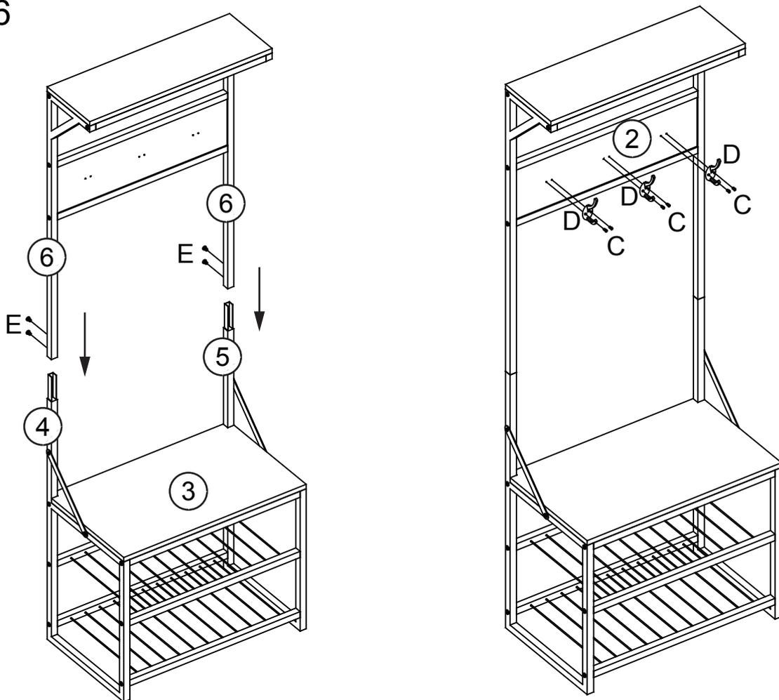
1. Place upper unit onto lower unit. Insert 4 machine screws (E) through holes on metal side frames (6), then tighten to secure upper unit to lower unit.
