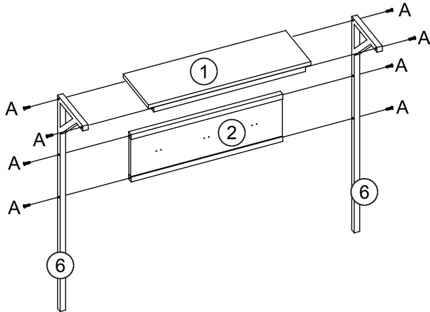
1. Attach 2 upper metal side frames (6) to top board (1) and back panel (2) by inserting 8 machine screws (A) through holes on upper metal side frames (6), then tighten to top board (1) and back panel (2).
