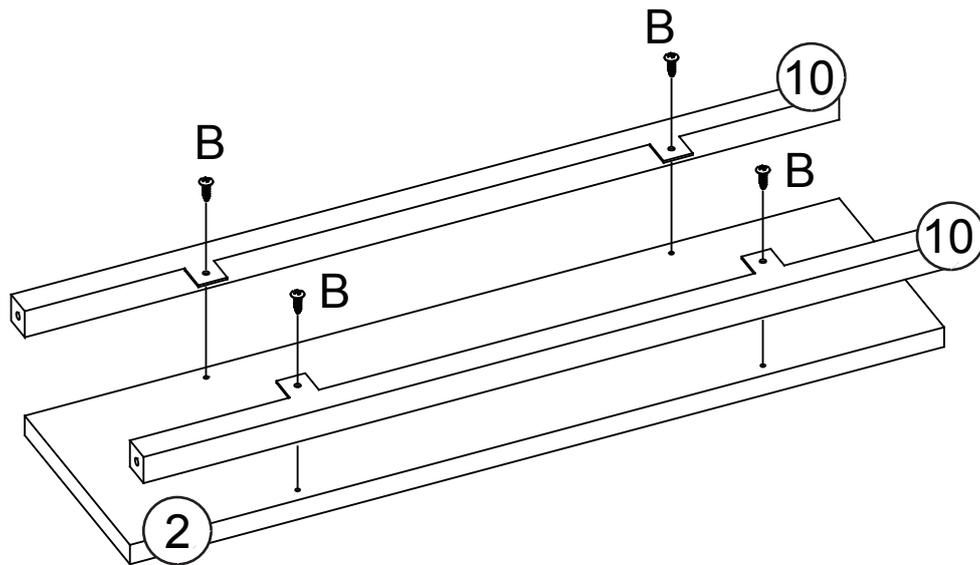
1. Attach 2 metal cross bars (10) to back panel (2) by inserting 4 screws (B) through holes on metal cross bars (10), then tighten to back panel (2).
