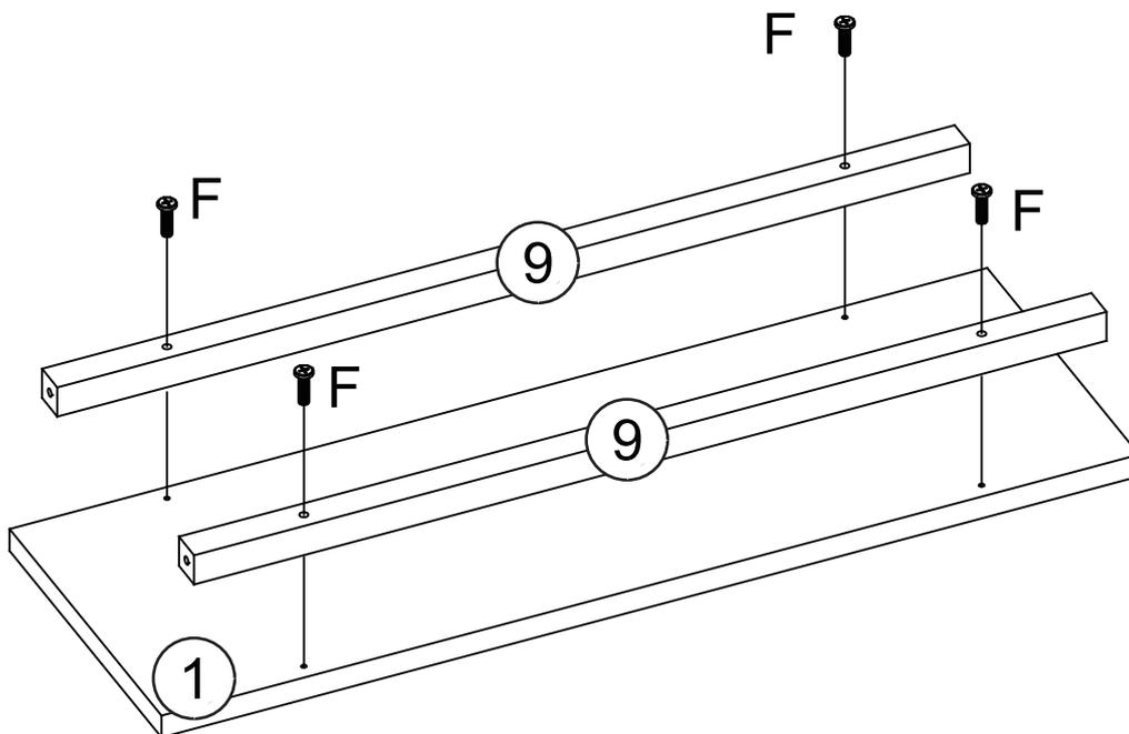
1. Attach 2 metal cross bars (9) to top board (1) by inserting 4 machine screws (F) through holes on metal cross bars (9), then tighten to top board (1).
