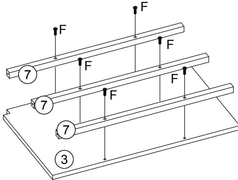
1. Attach 3 metal cross bars (7) to shelf (3) by inserting 6 machine screws (F) through holes on metal cross bars (7), then tighten to shelf (3).
