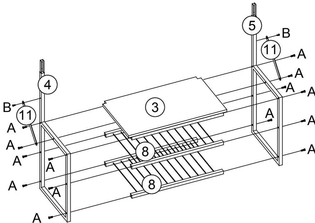
1. Attach lower left side frame (4) and support bar (11) to shelf (3) and bottom metal frames (8) by inserting 7 machine screws (A) and screw (B) through holes on lower left side frame (4) and support bar (11), then tighten to shelf (3) and bottom metal frame (8).
