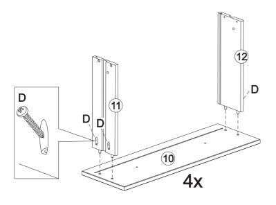
Attach parts (11,12) to part (10), insert panel (13) into groves and secure part (14) with screws(D) Insert knob (H) with screws(E).
