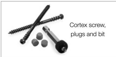
Use one Cortex screw per deck board to limit the movement of the deck board against the joist. The Cortex screw should be placed into the joist closest to the mid-point of each deck board from one end to the other end, and be centered on the deck board from side-to-side. This helps to ensure the deck board stays positioned as the environmental temperatures expand and contract the deck board.
