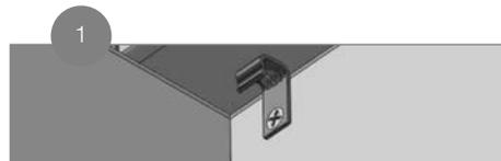
After positioning the last deck board in place, secure the deck board by angling a screw through the clip and into the board at a 30° - 45° angle. Be careful to make sure the screw inserts fully and pulls the board down (2). Space no more than 12 in. (30 cm) apart.
