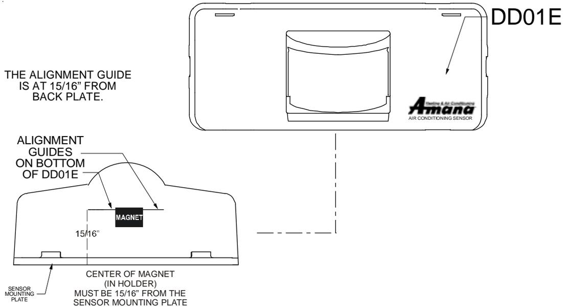
**IMPORTANT NOTE:** When properly installed, the center line mark on the bottom of the DD01E will line up with the center of the line of the magnet holder containing the magnet. Choose magnet position A, B, or C to align the magnet 15/16" from the back of the DD01E.
