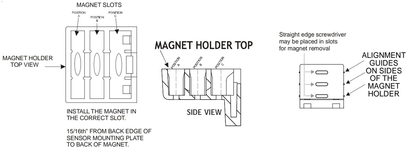
Select one of the three slots that places the magnet 15/16" from the sensor mounting plate on the door frame. See *following examples*. The door frame and door usually will not align. Place holder on the door and select the slot that places the magnet as close as possible to the 15/16" depth from the back of the DD01E mounting plate.
