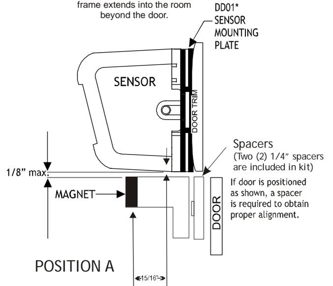
ABOVE SHOWS MAGNET 15/16" FROM THE SENSOR MOUNTING PLATE IN DIFFERENT SLOT POSITIONS
