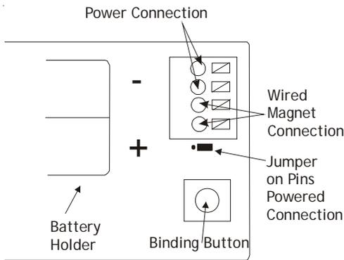
Note: For 24v powered connection, the jumper must be placed as shown above
