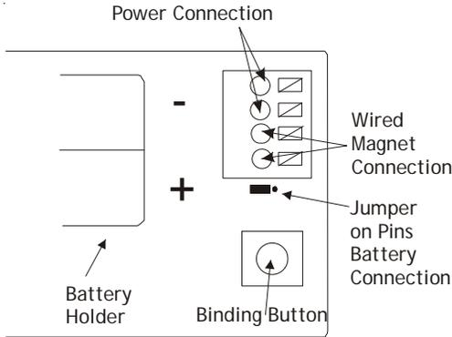
Note: For battery connection, the jumper must be placed as shown above
