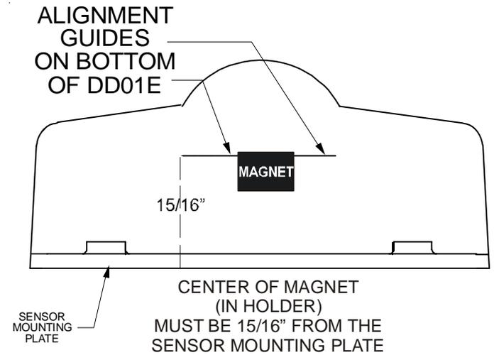
Do NOT install batteries until you are ready to test the magnet location with DD01E.
