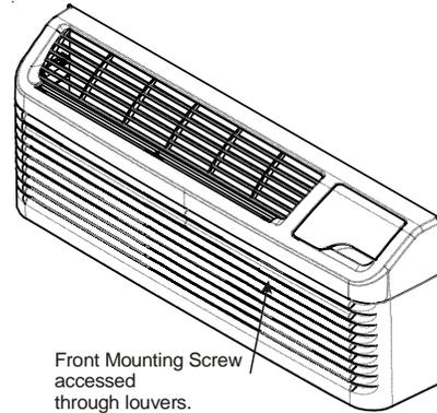
3. Remove cabinet front from chassis by tilting the bottom of the front forward, lifting slightly up and forward.
