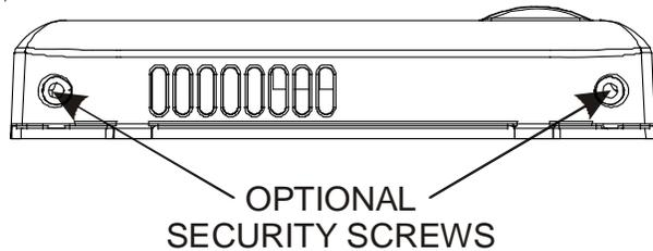
7. Snap motion sensor onto motion sensor mounting plate.
