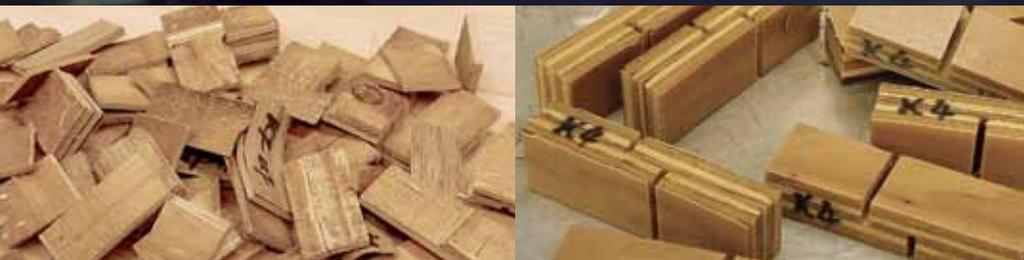
**Left to Right:** Traditional UF plywood after ANSI HP-1-2004 cyclic boil test, and PureBond plywood after the same test. PureBond's superior moisture resistance approaches Type I or waterproof performance: a quality rare in a decorative panel.
